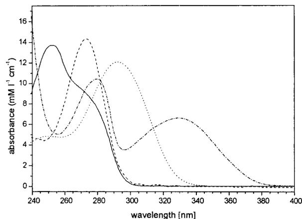
**Figure 6.** Ultraviolet spectra of compounds occurring in the reaction trajectory of GTP cyclohydrolase I.<sup>11</sup> (—) GTP (compound 1); (---) 2-amino-5-formylamino-6-ribosylamino-4(3H)-pyrimidinone 5'-triphosphate (compound 4); (·····) 2,5-diamino-6-ribitylamino-4(3H)-pyrimidinone 5'-monophosphate (compound 5-monophosphate); (-·-·-) dihydroneopterin (the triphosphate isomer compound 10).
