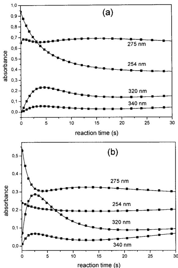
**Figure 7.** Absorbance changes obtained from single turnover stopped-flow experiment with wild-type GTP cyclohydrolase I and GTP (a), resp. compound **4** (b). Symbols represents the original data, lines represents the data obtained from numerical simulation using the kinetic constants in Table 1.
