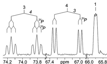
**FIGURE 4.**  $^{13}\text{C}$  NMR signals of  $[1,3,4\text{-}^{13}\text{C}_3]\text{4-diphosphocytidyl-2C-methyl-D-erythritol 2-phosphate (6)}$ . Coupling patterns are indicated.
